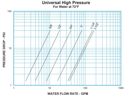
**Note:** All flow curves and Cv values presume the valves are fully open with 1/2 PSI cracking pressure springs. Consult the factory for more information.
