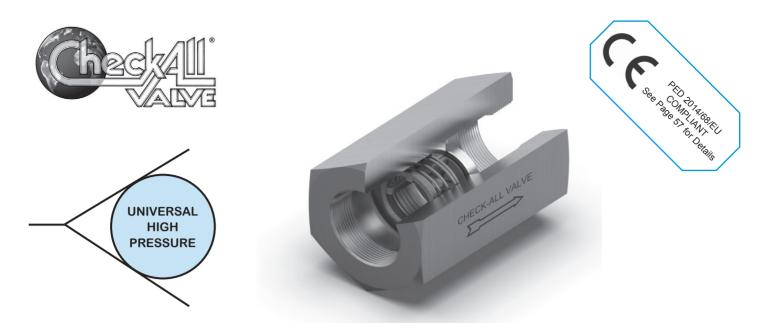
The **Universal High Pressure (U1, R1)** check valve is a one piece body machined from bar stock with female pipe threads. The valve is designed and manufactured for high pressure applications. These valves can also be used as low pressure relief valves or vacuum breakers by using the desired spring settings. This valve is normally supplied with a "metal-to-metal" seat. NPT threads are per ASME B1.20.1. Also available with ISO 7 "Rp" threads (R1).
